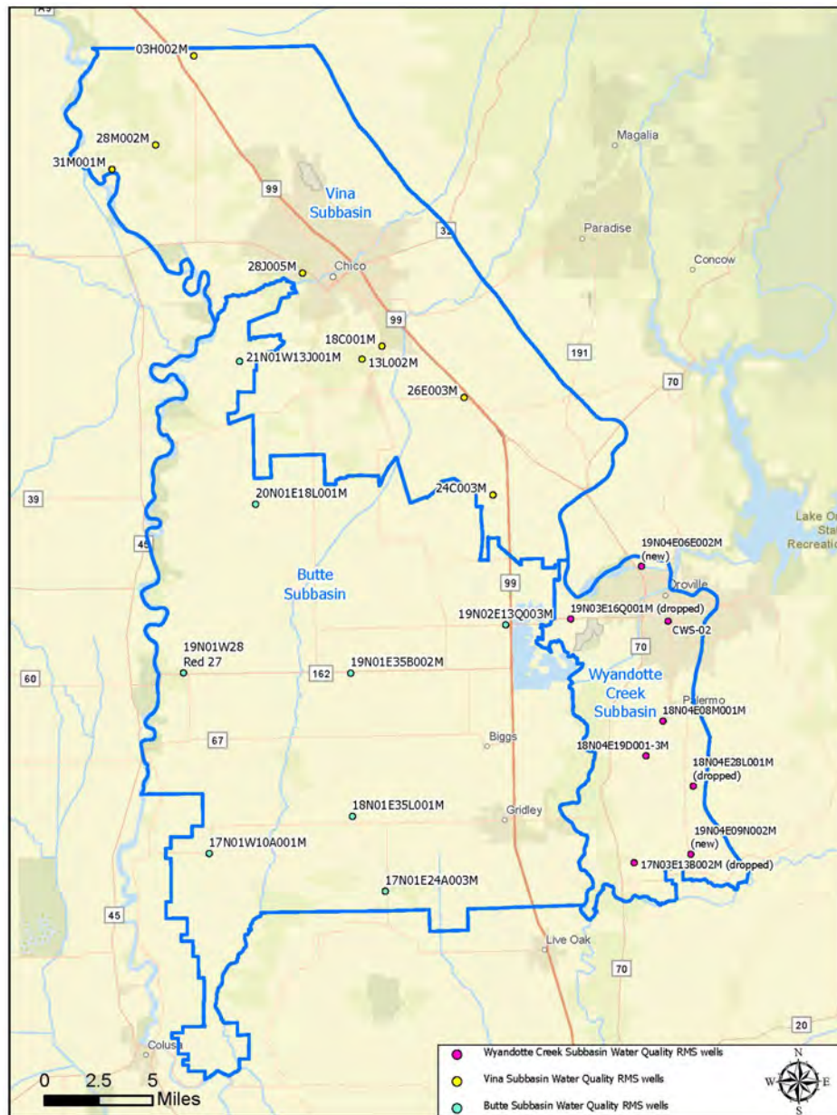
Figure 1. Groundwater Quality Representative Monitoring Site well locations in the Vina, Butte and Wyandotte Creek Subbasins
