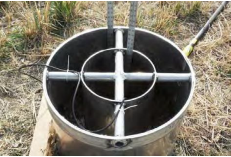
Photograph 3. Double Ring Infiltrometer
