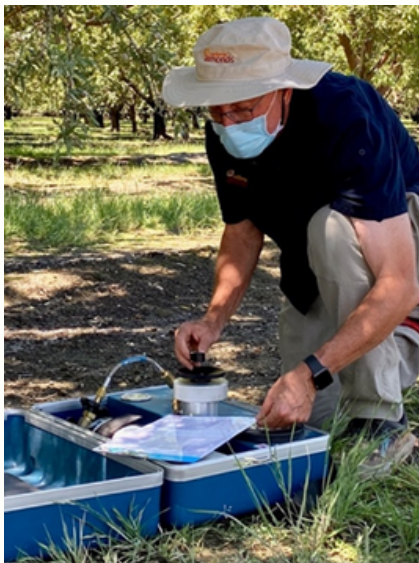
Figure 6. Pressure chamber in use.
